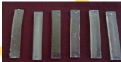
Figure 5. Specimens for three points bend test.
