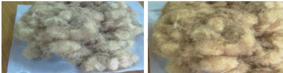
Figure 2 Treated chopped Sisal and Banana fibres
