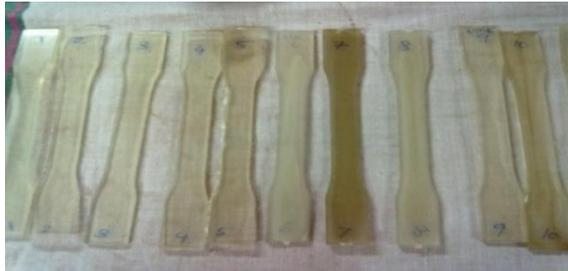
Figure 4. Tensile test specimens
