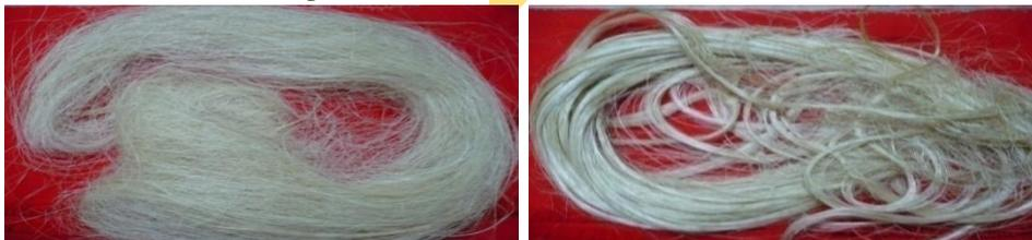
Figure 1 Untreated Sisal fibre & Banana fibre
