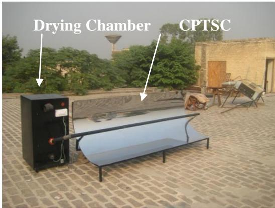
**Figure 1: Concentrating Parabolic Trough Solar Collector.**
